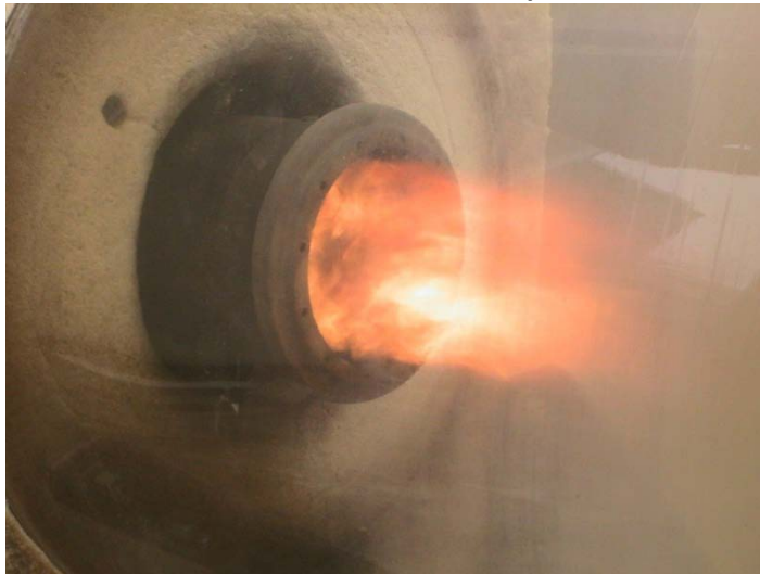
Figure 14) FFA fuel (processed trap grease) firing in a residential oil burner in tests at Brookhaven National Lab. Fuel temperature is 230 F.
